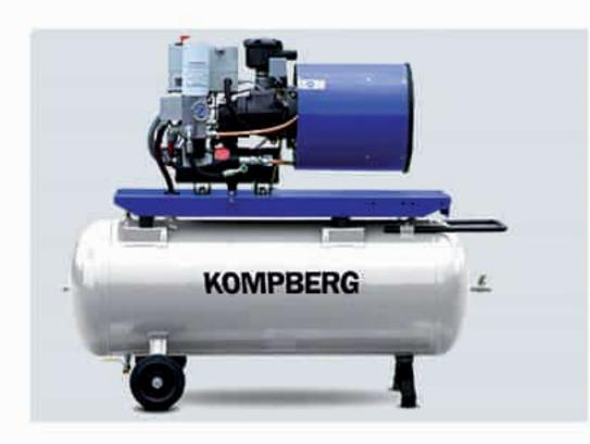
Compressor output is controlled either as for piston compressors by an on/off switch, depending on the pressure in the air chamber or by classic suction regulator with a new control system depending on the pressure level, or possibly by advanced continuous regulation of operation, which optimises the machine's performance parameters in real time by smoothly changing revolutions depending on the volume of discharged compressed air
